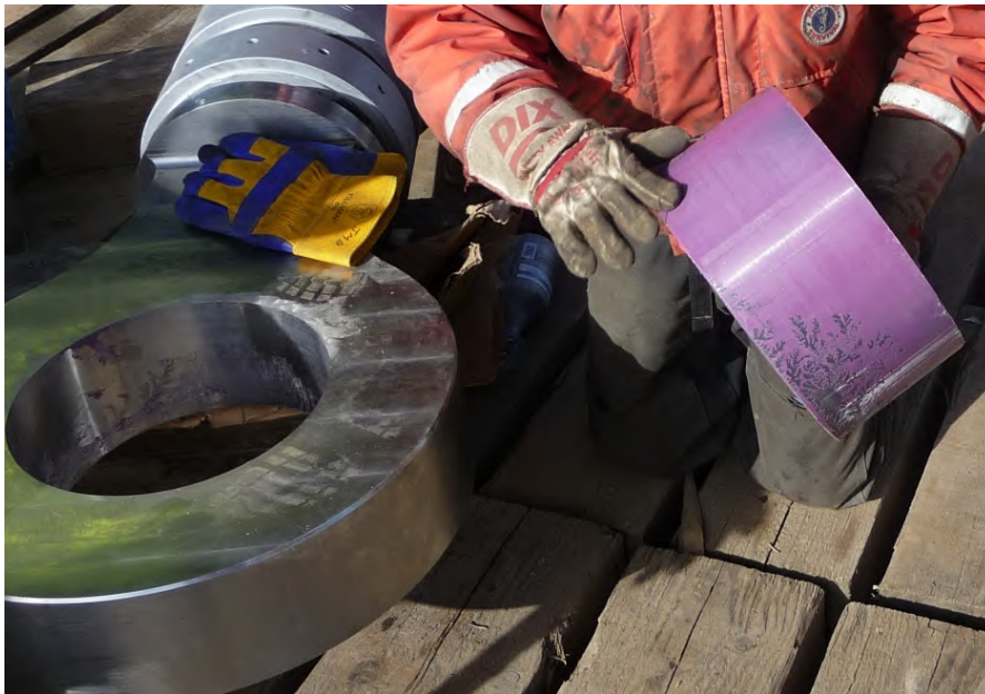
Figure 12-17. Disbonding Failure from Improper Housing Surface Preparation.
