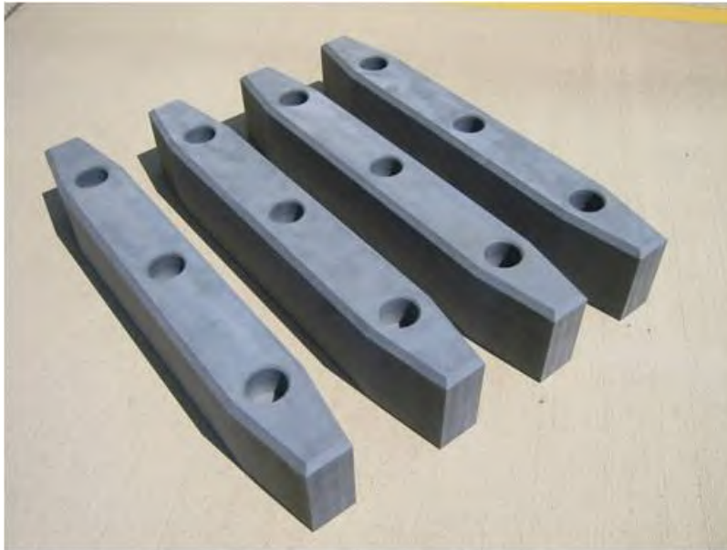
Figure 12-31. Vertical Lift Gate Guide Blocks.
